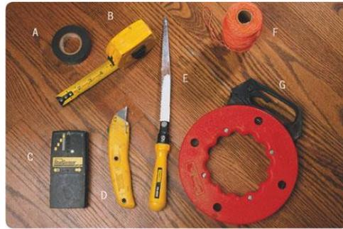
Here are some of the tools you may need for your project: (A) electrical tape; (B) measuring tape; (C) a stud finder; (D) a utility knife; (E) a drywall saw; (F) string (for pulling wire short distances); (G) a fish tape (for pulling wire longer distances).
